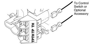
Figure 45 - Control Valve Terminals
